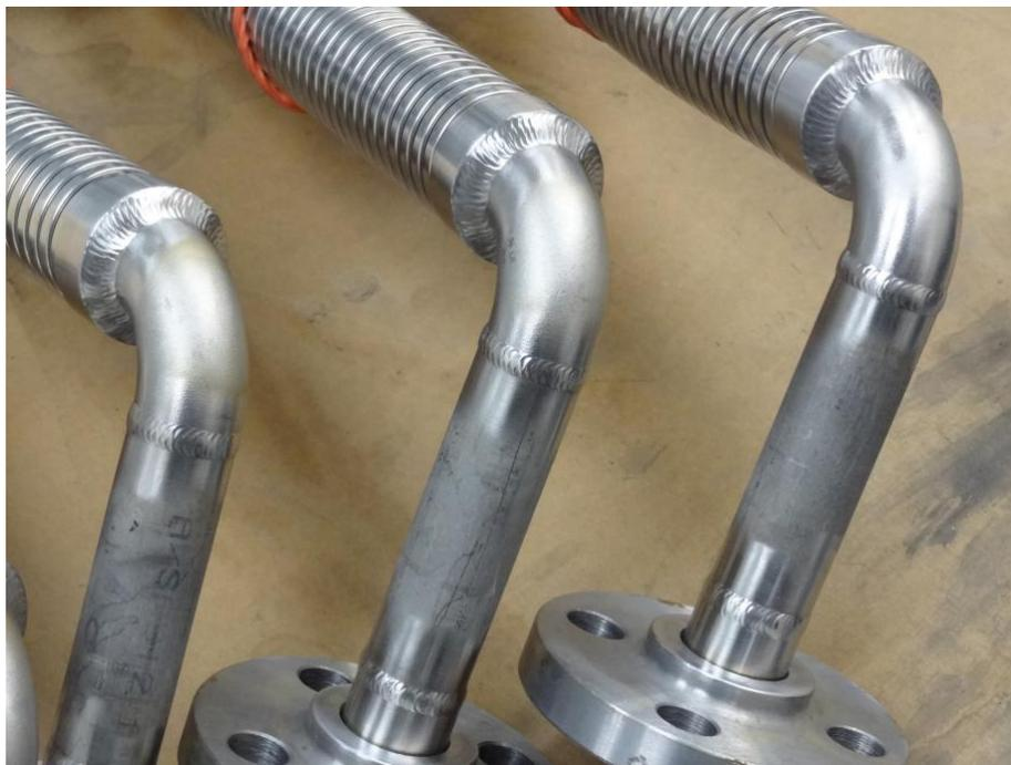
At the other end of the spectrum, grey coloring is often accompanied by a rough surface, termed “gross oxidation” or “sugaring.” Differences in the quality of purged and unpurged welds can also be clearly seen when looking at the inside of the weld.
