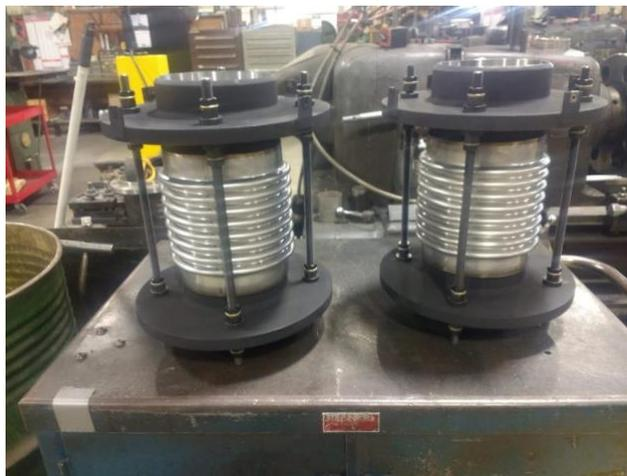
The number of limit rods is calculated based on the pressure thrust that needs to be contained. EJMA recommends a minimum of three rods.
