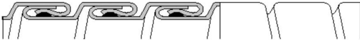
These days, when used alone, interlocked hoses convey small solid particles like grain or plastic pellets for injection molding machines. The packing is not tight enough to seal against leaks from a liquid.
