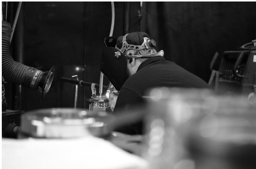
Penflex ASME Section IX welder performing cap pass on metal hose assembly.
