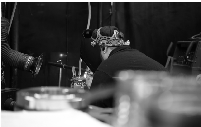
Penflex ASME Section IX welder performing cap pass on metal hose assembly.
