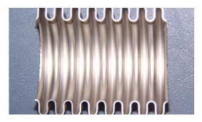
The object is to measure the material thickness at different locations along the tube to determine if the material thickness of the flat, rolled steel is maintained and consistent.
