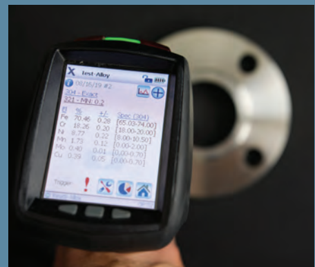
PMI analyzer reveals flange is 304 SS
