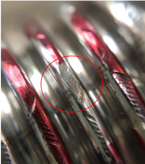
Figure 3: Crack in Annular Hose
