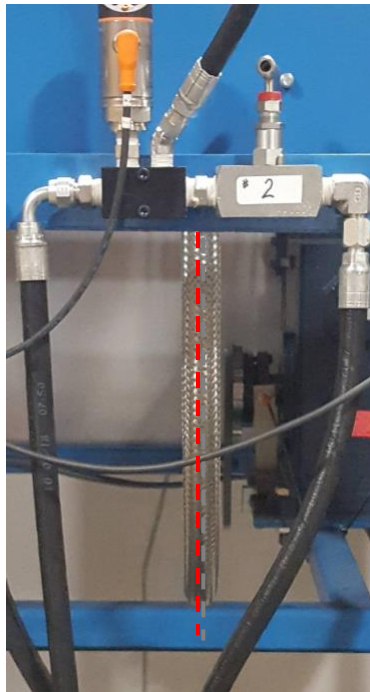
Figure 1: Annular hose at \approx 115,000 cycles
